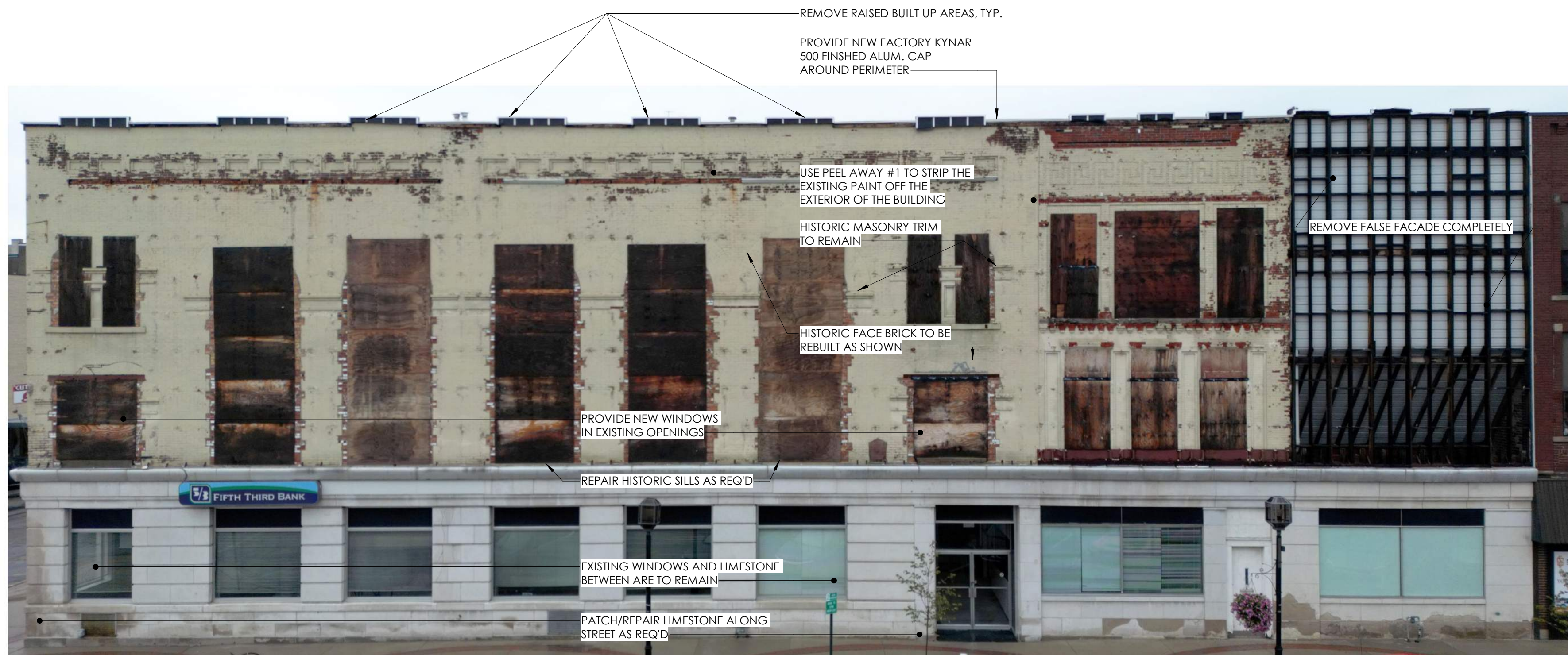
1 A502 ENLARGED NORTH ELEVATION 1/4" = 1'-0"
